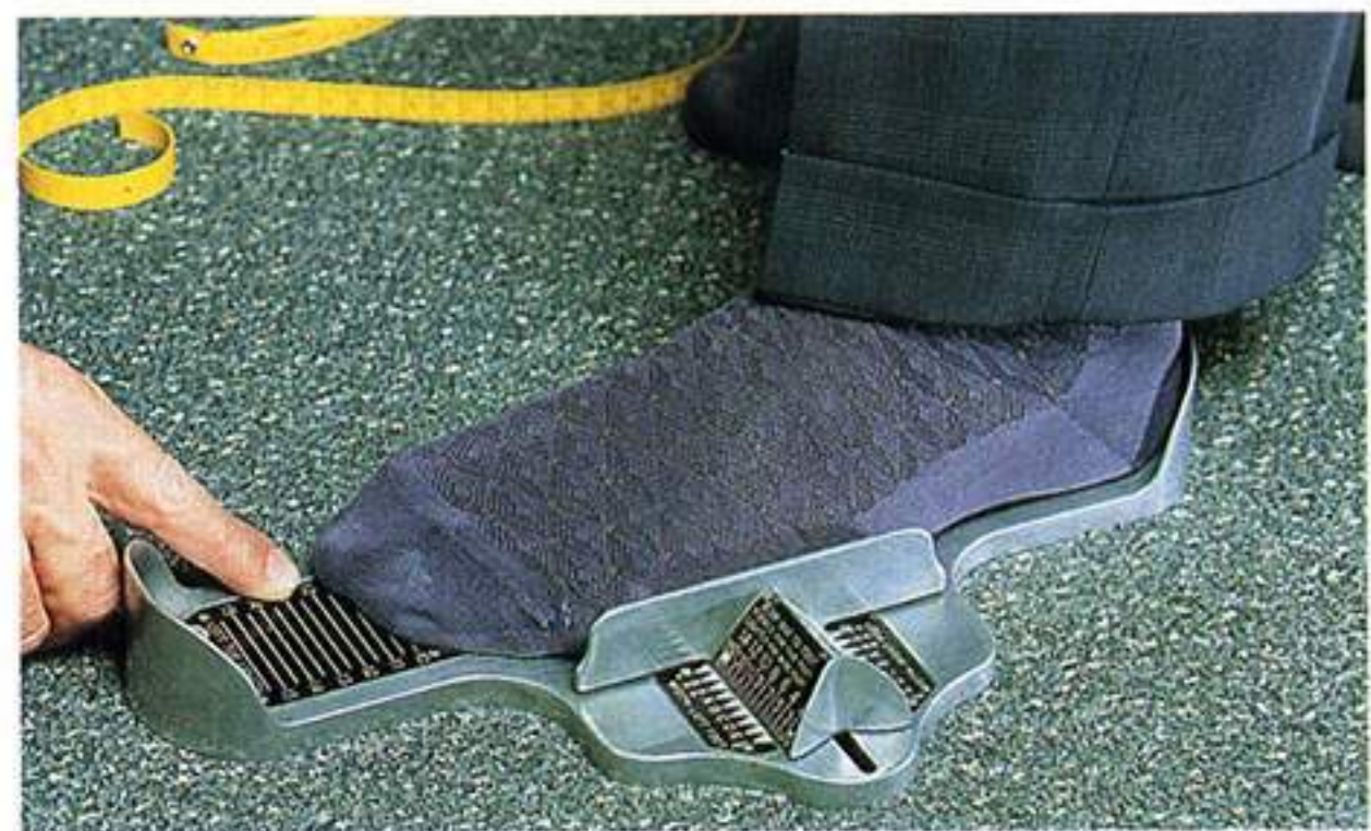
The foot must be placed on the device with the heel against the heel cup, and the toes pressed onto the base. The shoe size can then be read off correctly.
