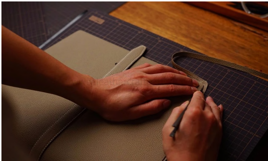
Step 60: Cut off redundant A20 part.
