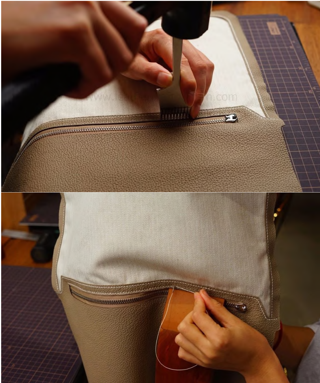
Step 51: Punch chisel holes and sew.
