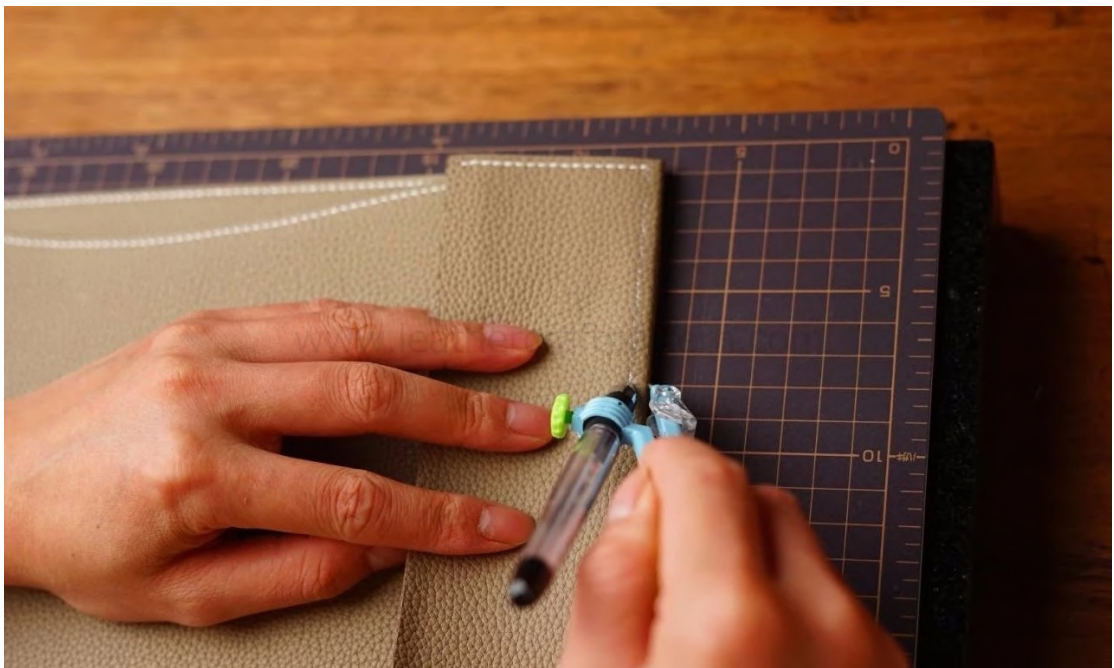
Step 97: Draw stitching line and punch chisel holes.
