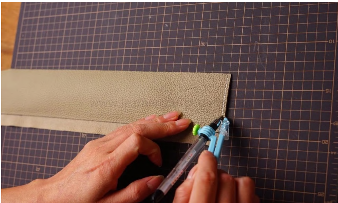
Step 88: Draw stitching line on short edge.
