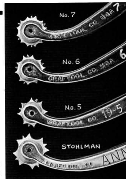
PHOTO ABOVE SHOWS THREE SIZES OF BUCKSTITCHING WHEELS MADE FROM CRAFT TOOL OVERSTRETCH WHEELS No. 5 - No. 6 - No. 7. . . . USING METHODS SHOWN AT LEFT. STOHLMAN WHEEL (ON PAGE 26) IS SLIGHTLY LARGER THAN THE No. 5.
