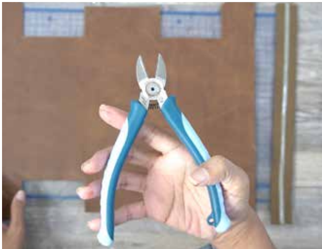
Use sharp tip plier to cut the zipper teeth
