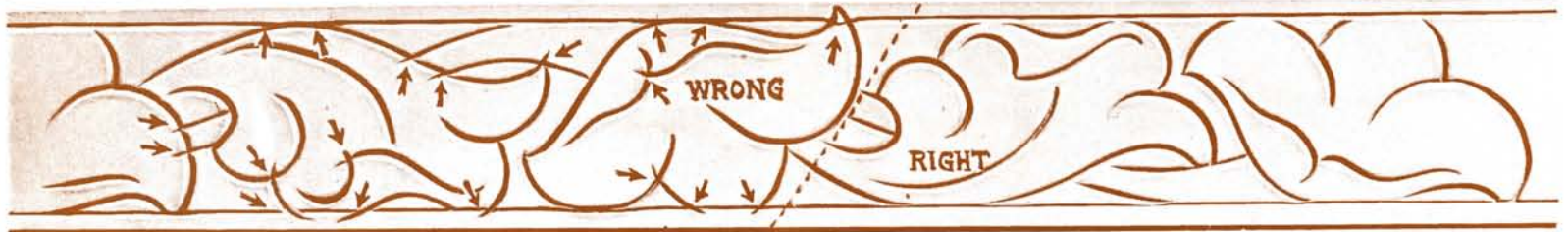
Fig. 4 Do not join cuts at intersecting or parallel lines (see arrows) as this leaves a sliver of leather that may stick up—use care!
