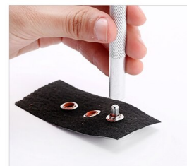
4. Put the install rod on washer, then hammer the eyelet and washer together.
