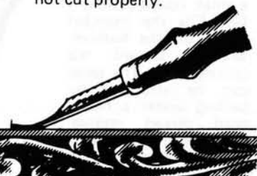
TOO SHALLOW Tool will skip; will not cut properly.
