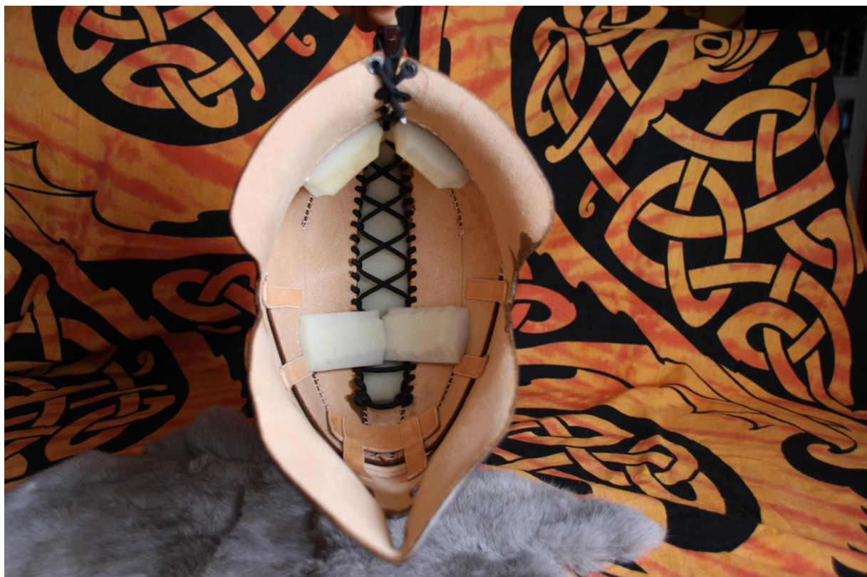
Figure 3: Zigzag pattern from the inside and foam
