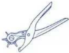
Multi-hole Punch A punch for punching holes of different sizes on leather.
