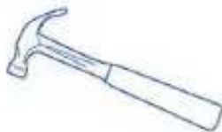
Hammer A small hammer used for setting rivets and eyelets.
