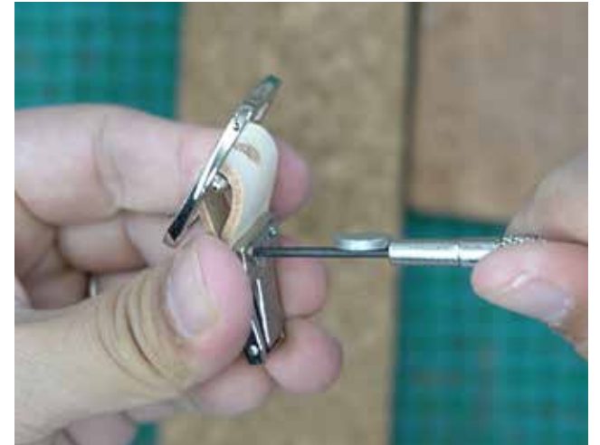
Install turn lock closure at the end of the fold
