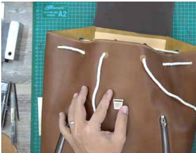
Install the turn lock closure to the body
