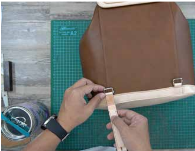
Slide the ends to rectangle ring and stitch to lock
