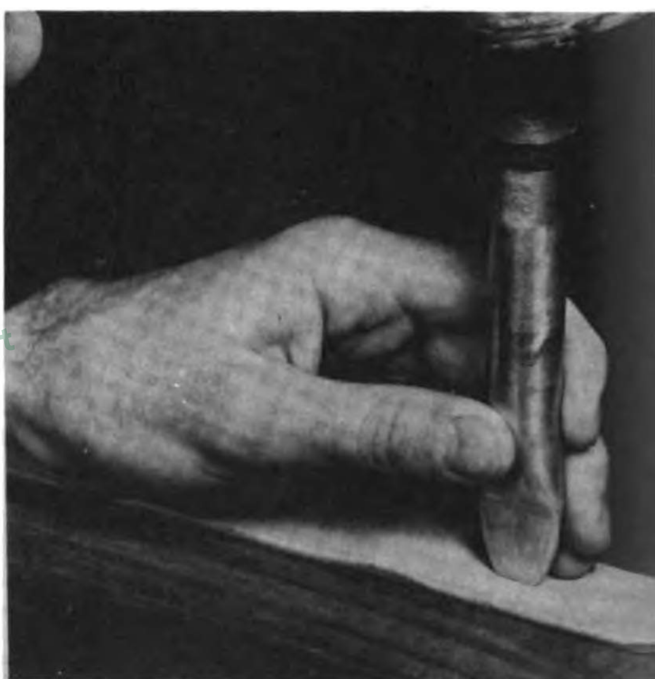
135. Punching an Oblong Hole for a Belt Buckle
