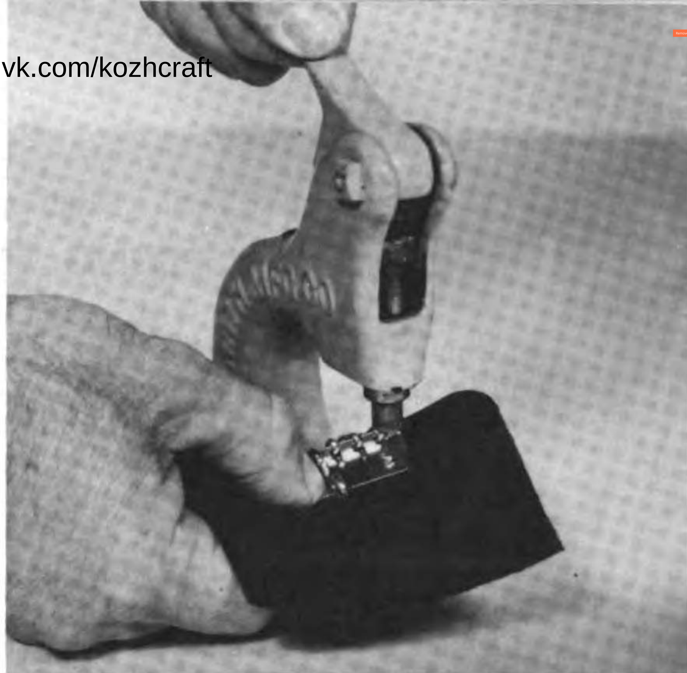
137. Setting an Eyelet with a Hand Lever Eyelet Setter
