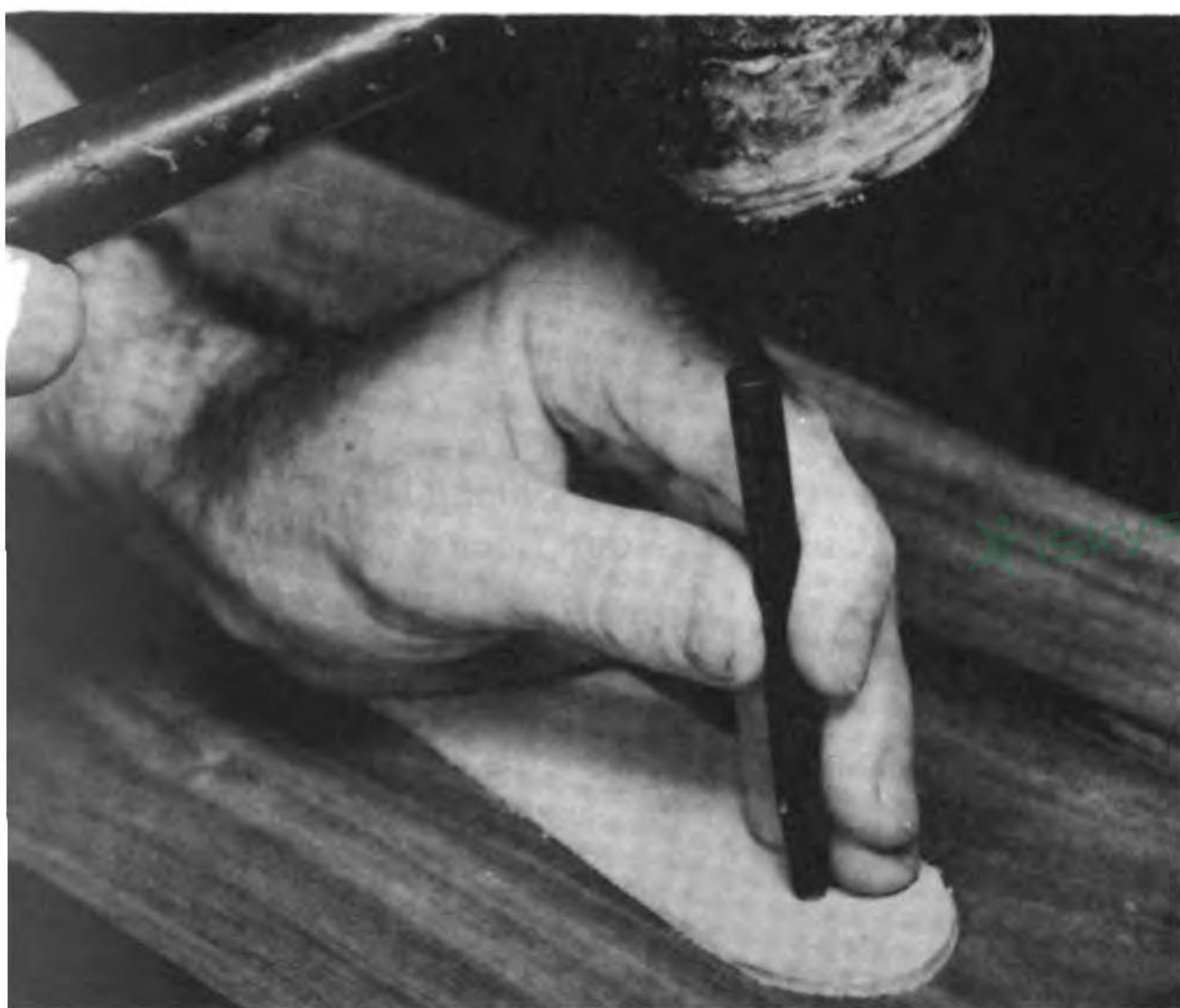
133. Punching a Hole with a Hollow Drive Punch
