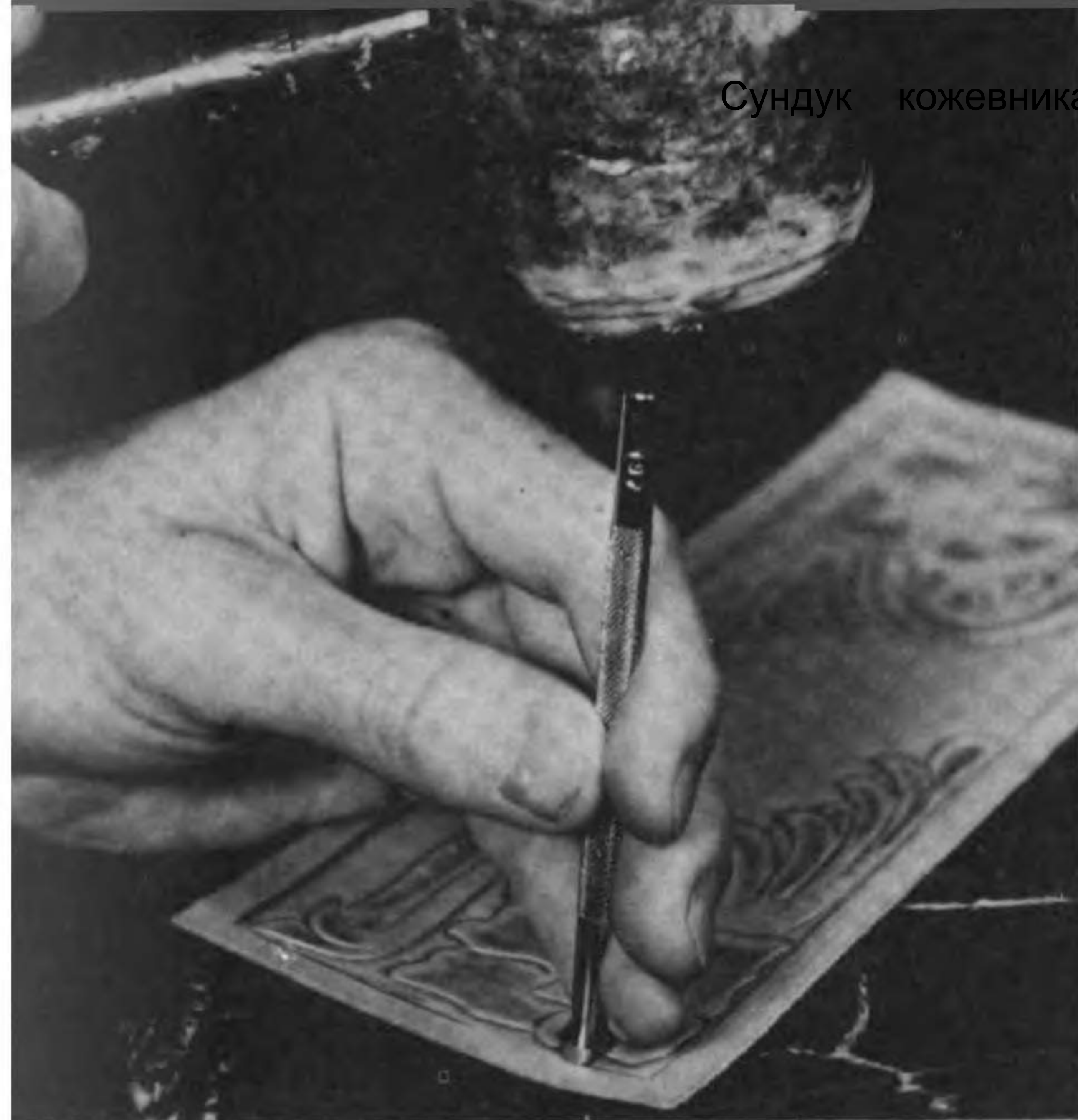
84. Beveling Produces a Depth Dimension
