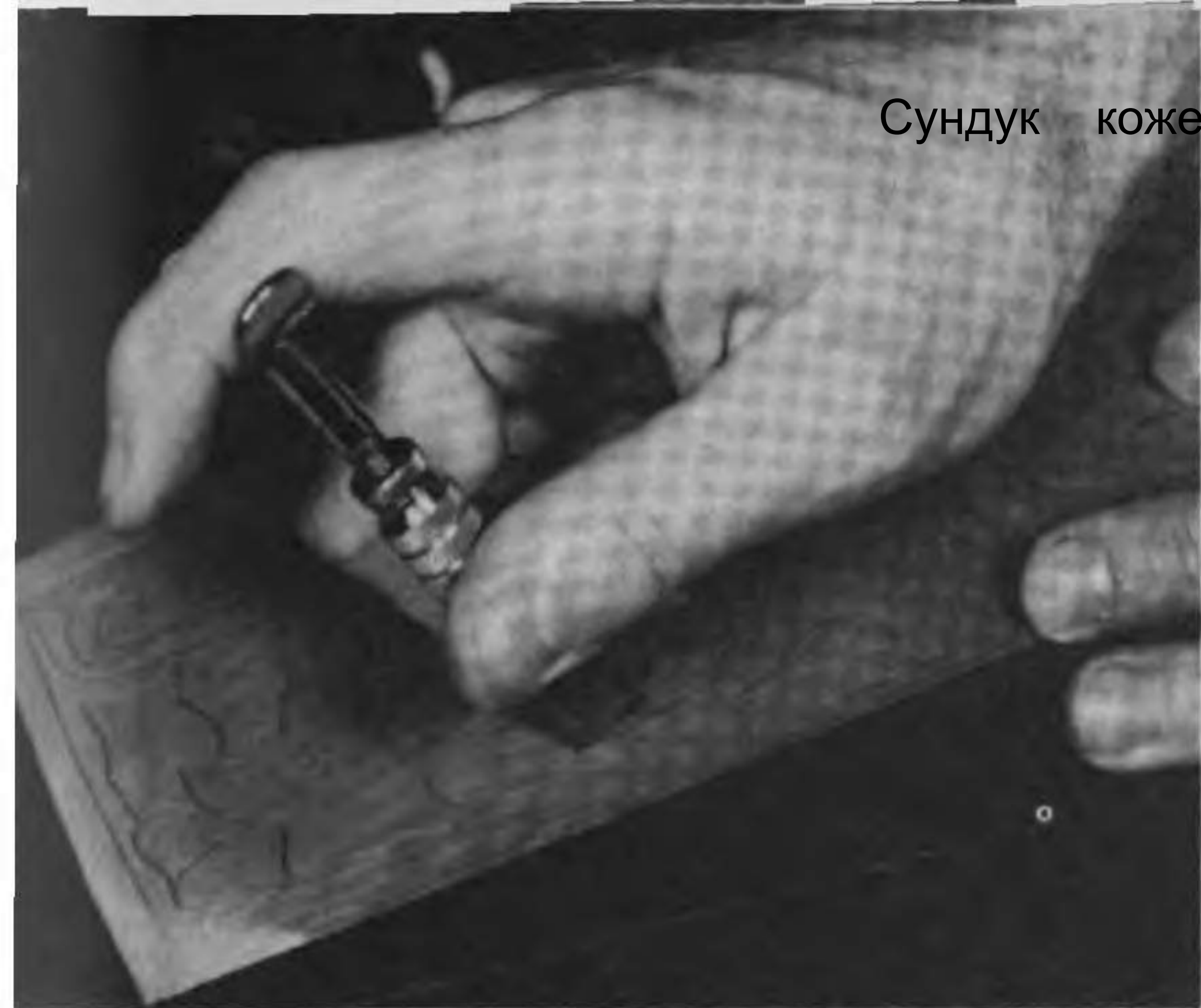
76. Carving or Cutting the Outline of the Design with a Swivel Cutter
