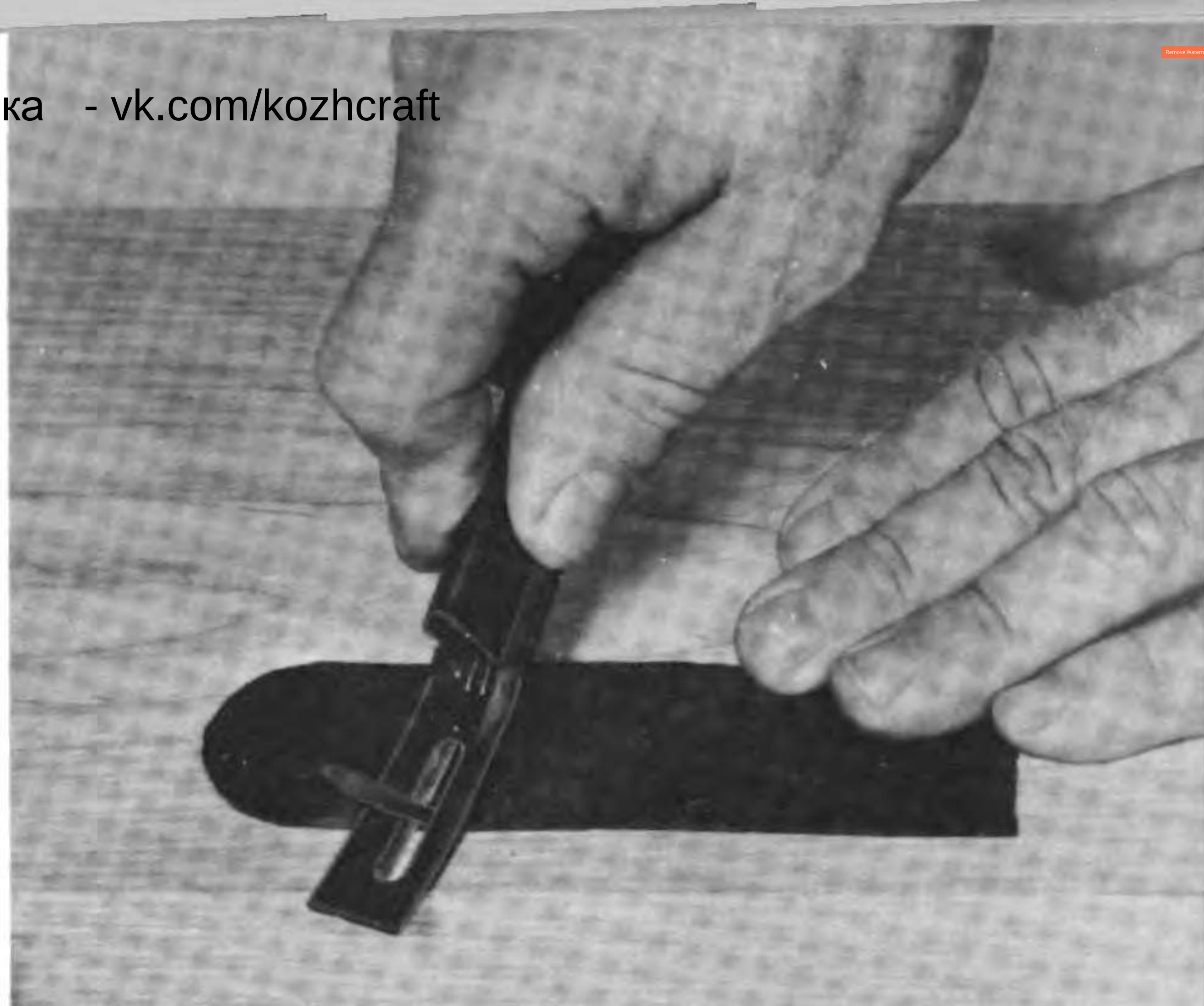
93. Skiving the Edge of a Comb Case with a Skife
