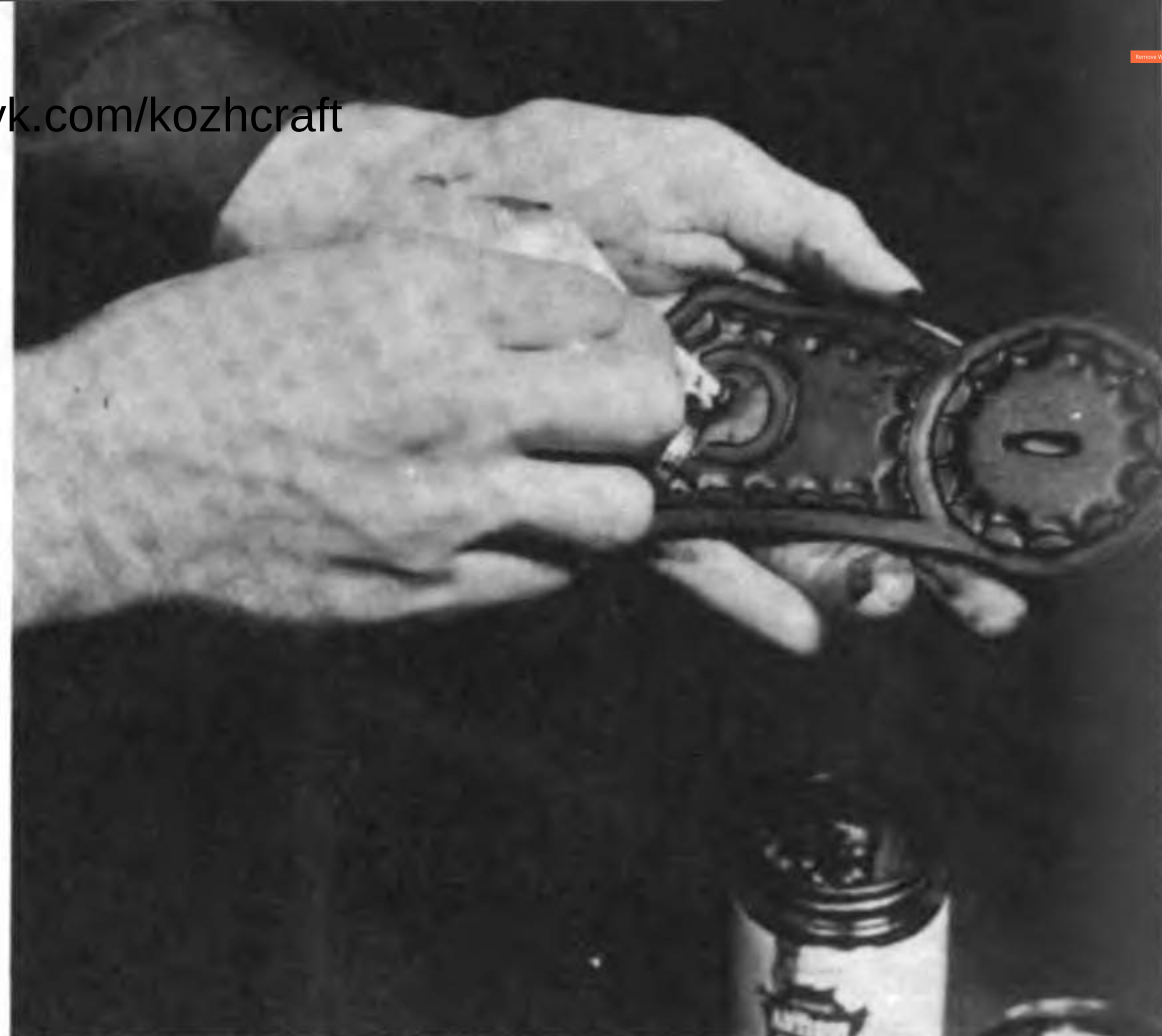
158. Removing Excess Antique Paste or Cream from the Leather Surface
