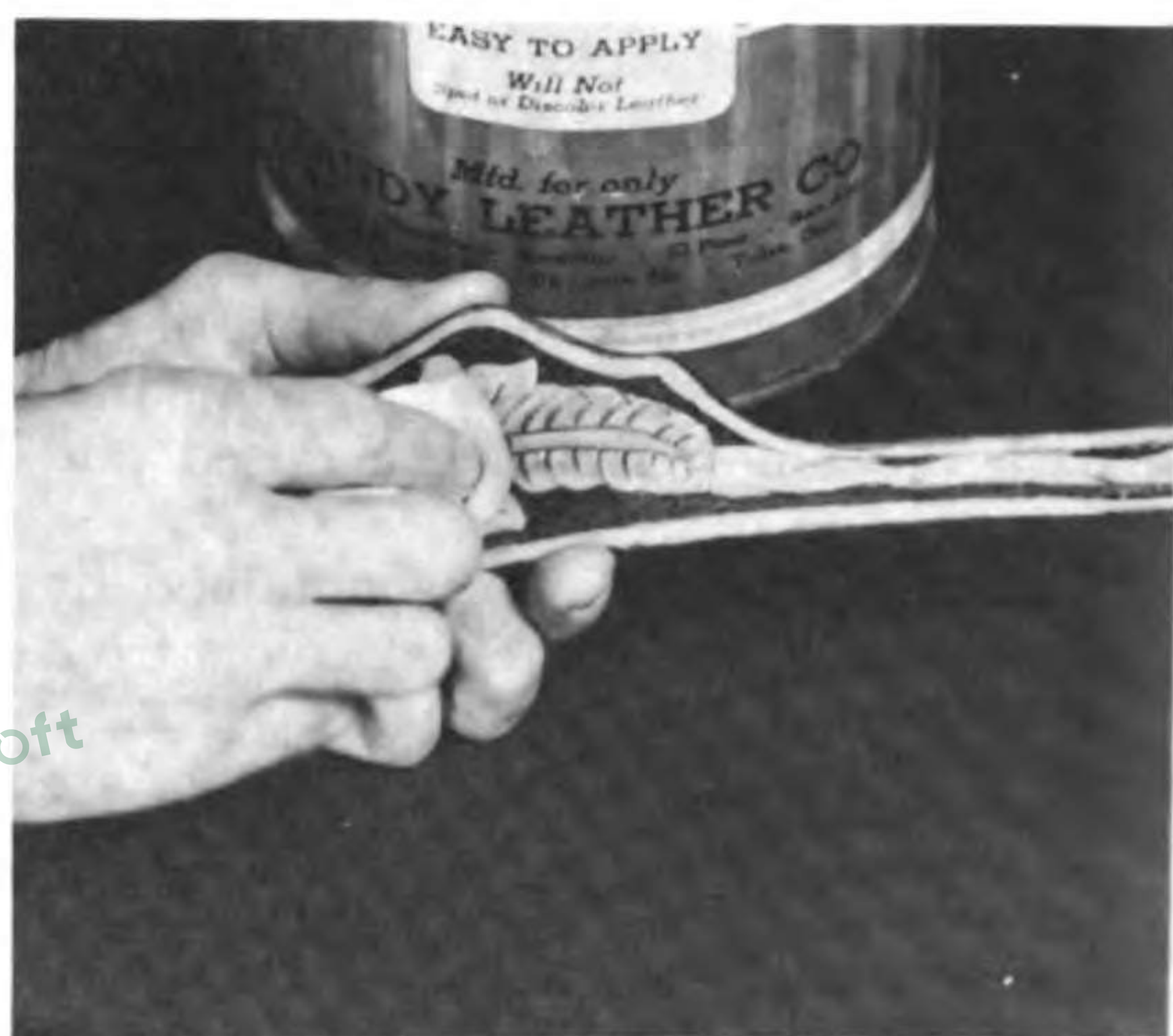
159. Applying a Coat of Clear Leather Lacquer Protects the Finish
