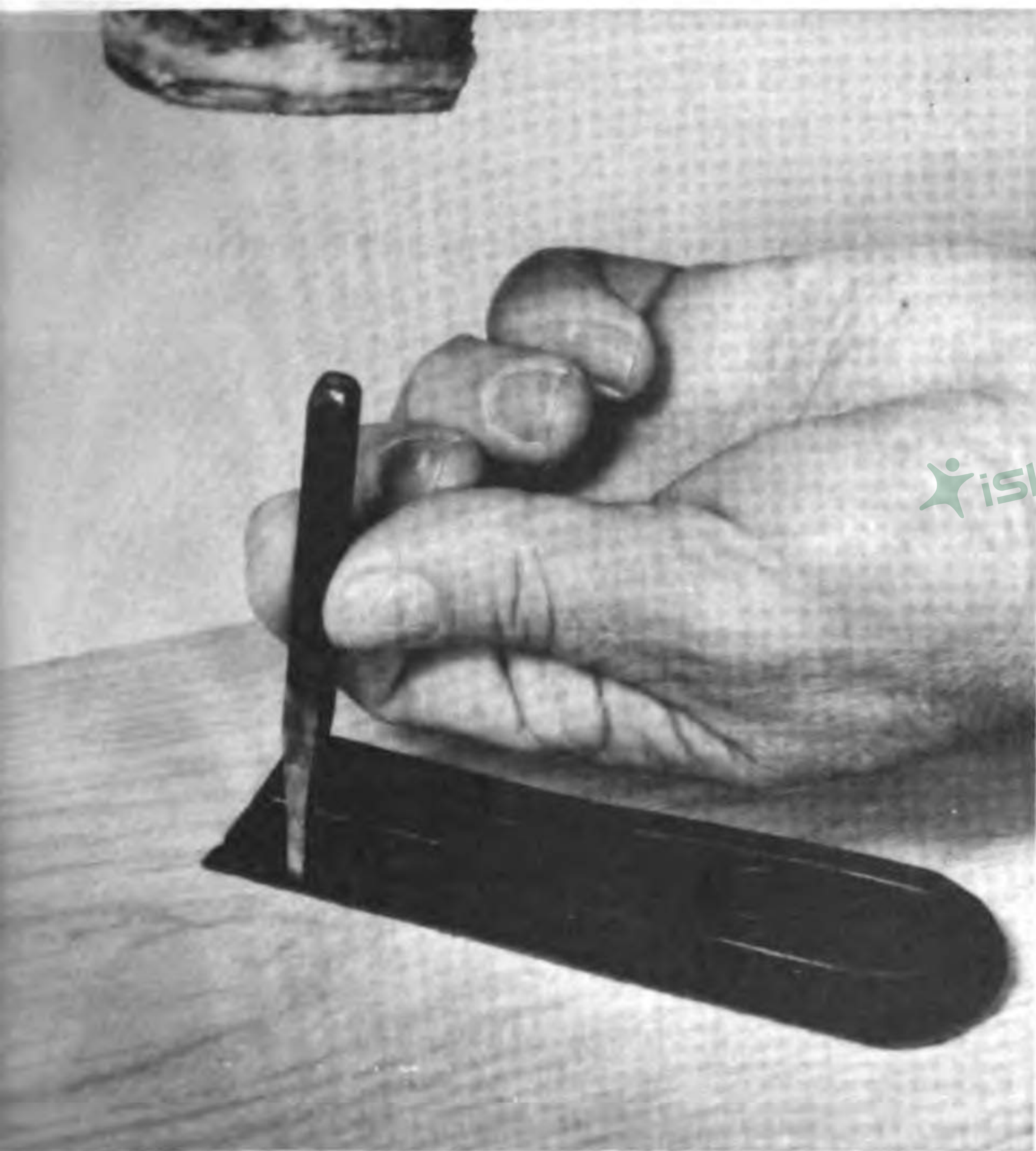
112. Driving a One Prong Chisel to Make Thong Slits
