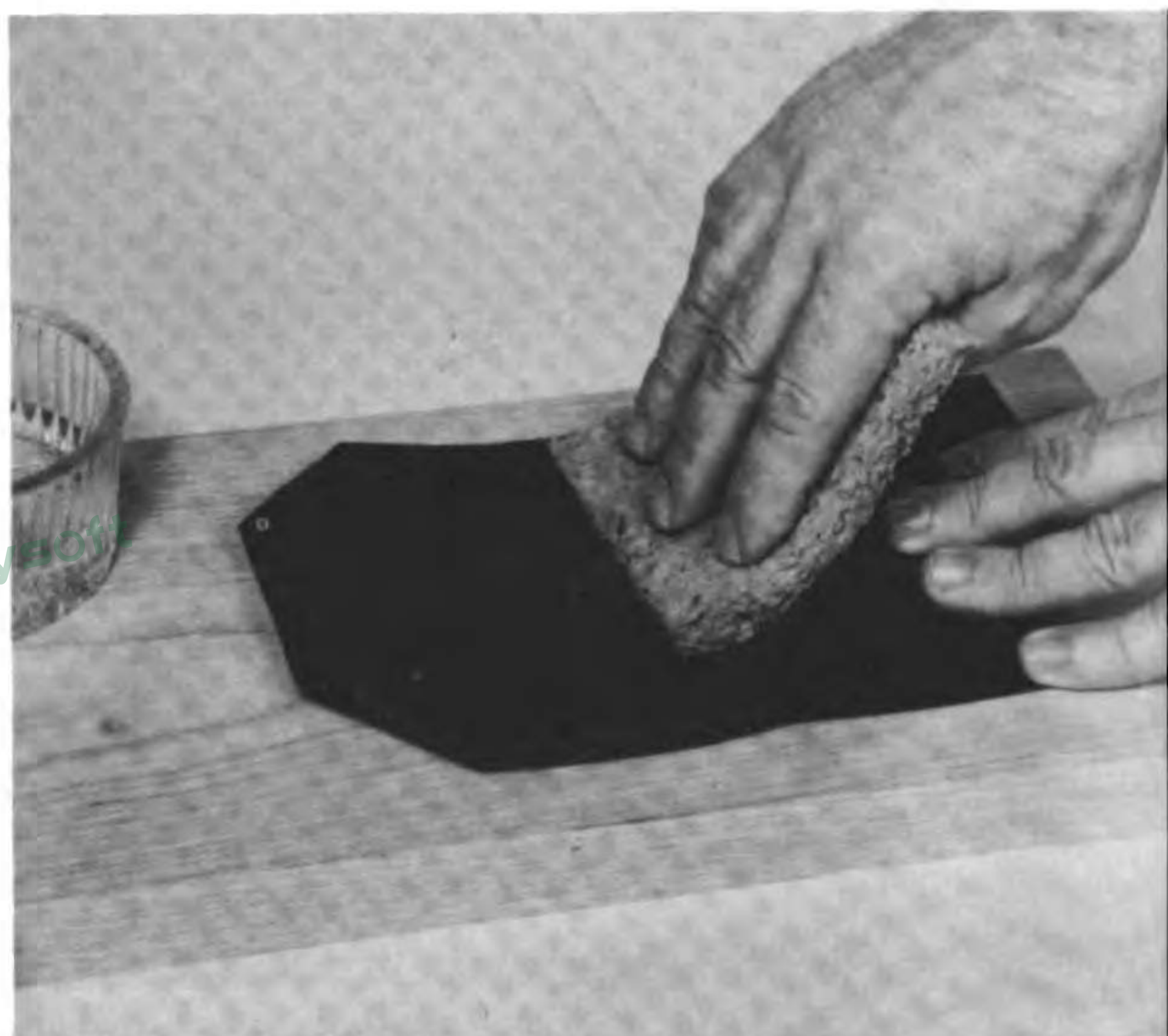
57. Moistening the Rough or Flesh Side of Light Weight Leather before Transferring the Design and Tooling
