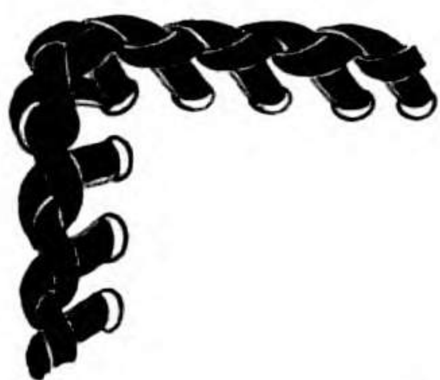
125. Rounding a Corner with the Single Cordovan Edge Lacing
