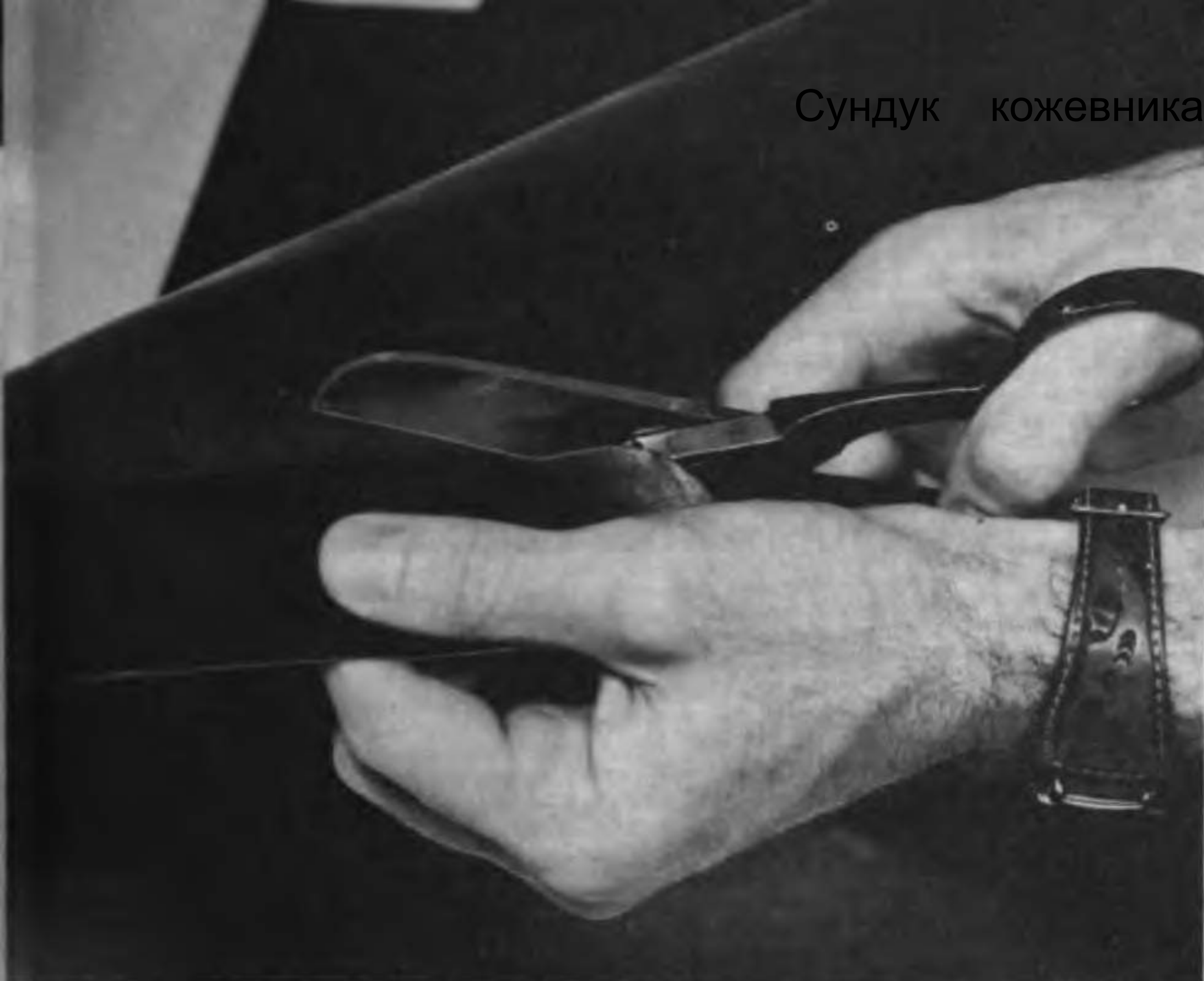
51. Cutting Light Weight Leather with a Serrated Edge Leather Scissors
