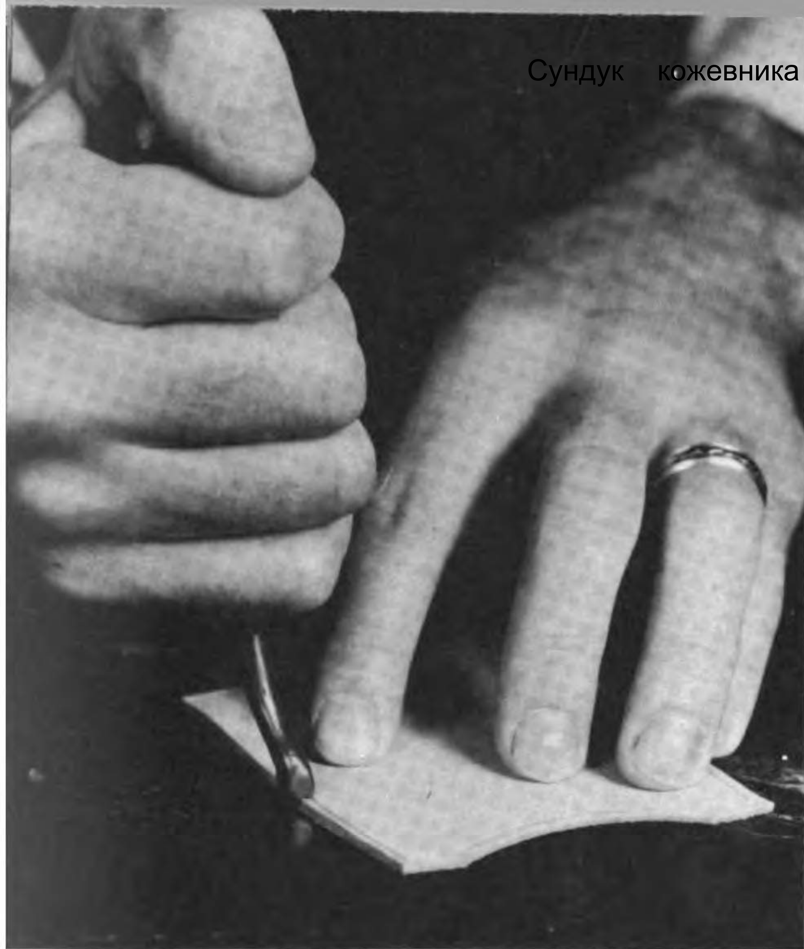
95. Creasing the Edge of a Belt with a Metal Edge Creaser
