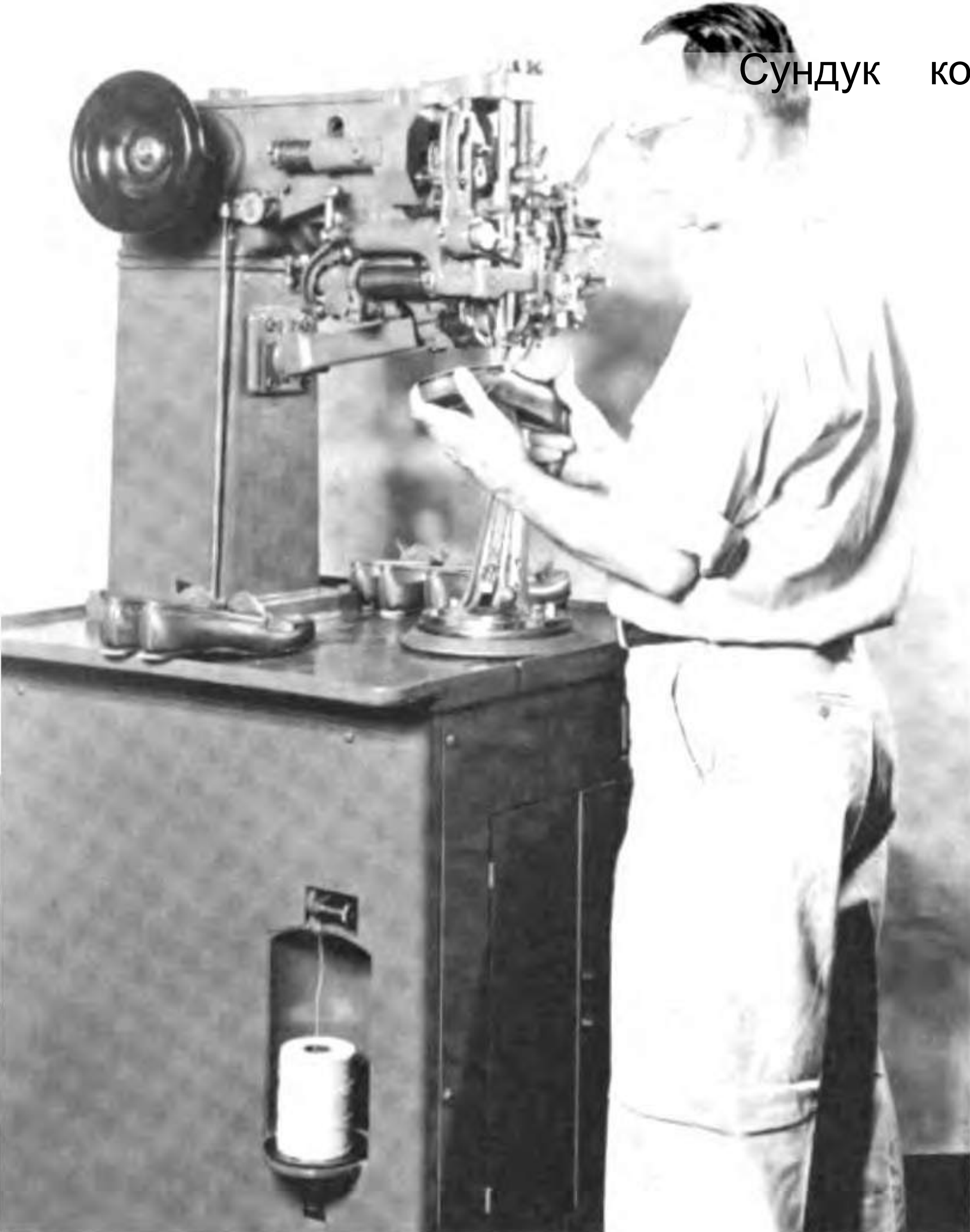
223. Sole Stitching Machine. This Machine Lockstitches Outsoles, Platforms, Midsoles, and Taps
