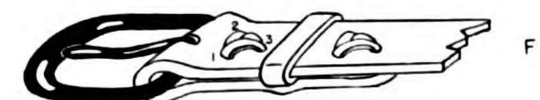
145. Detail of Three Hole Fastener
