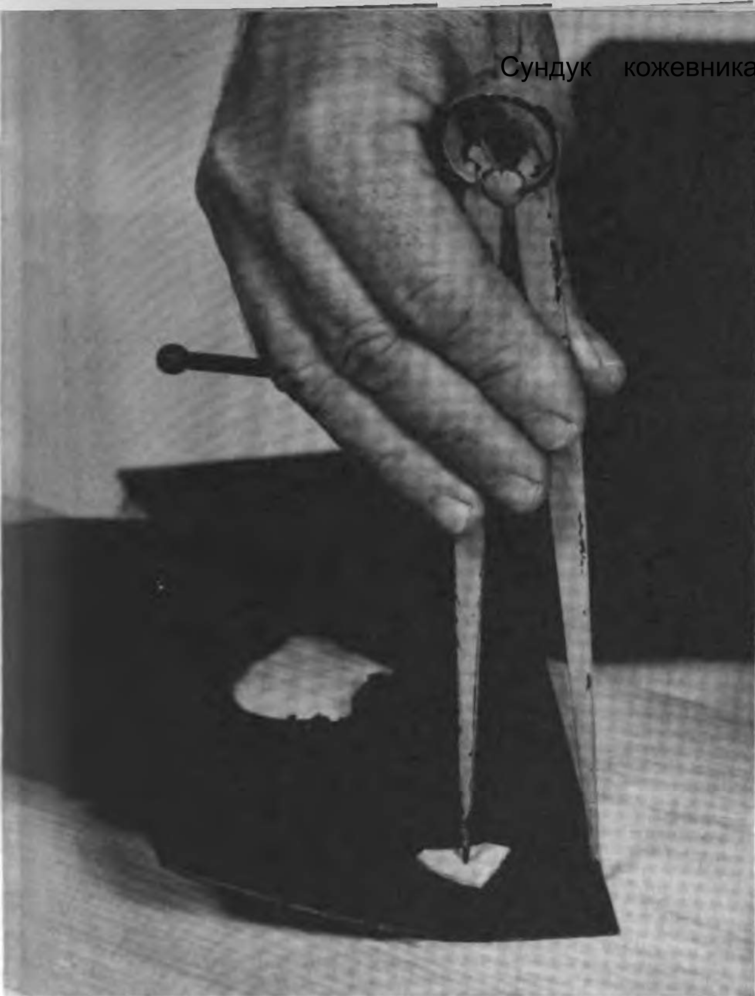
47. A Radius May Be Inscribed on Leather with a Dividers. Note the Center Is Placed on a Piece of Heavy Cardboard or Piece of Scrap Leather to Avoid Injury to the Leather
