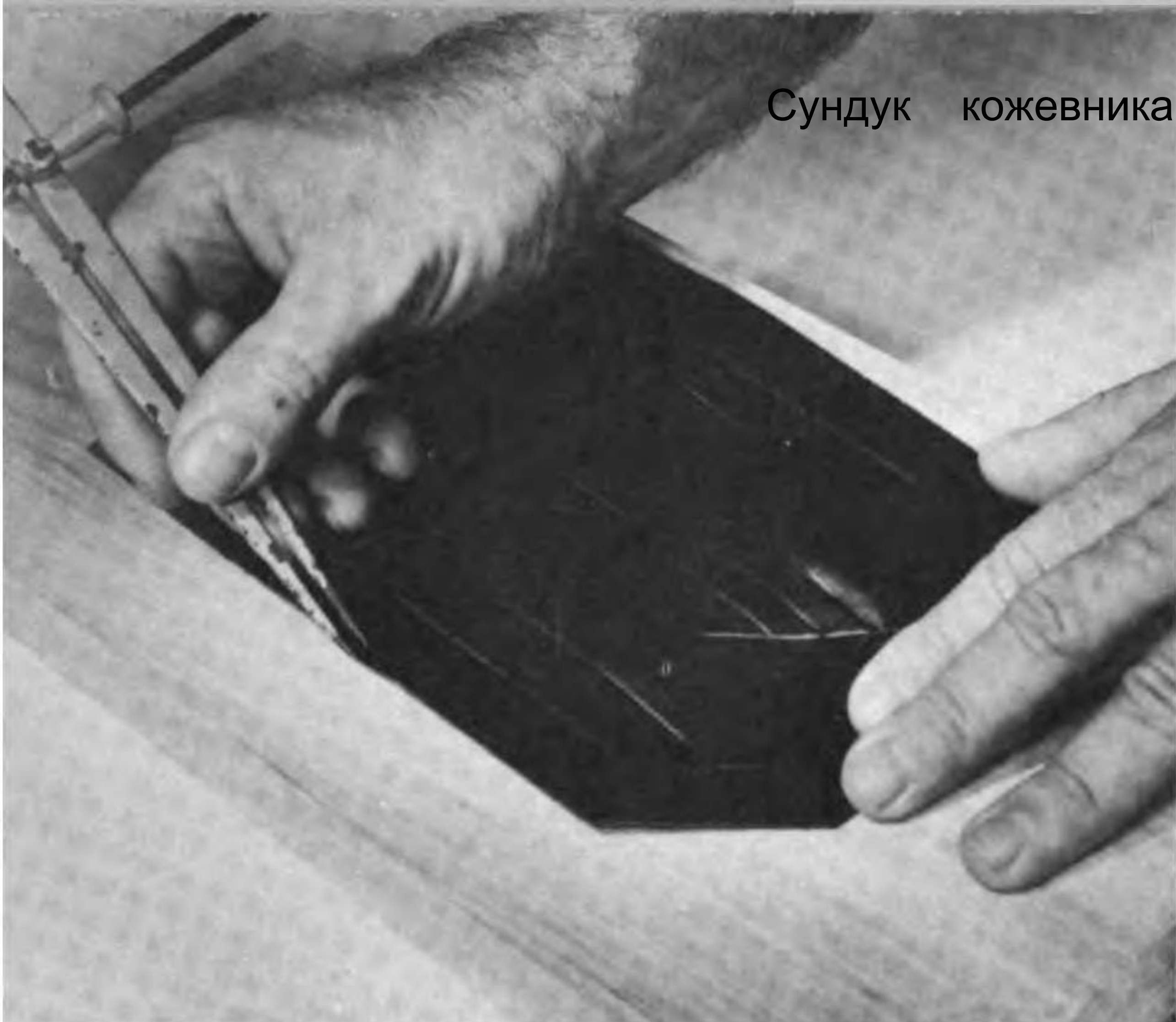
109. Marking Lightly the Gauge Line for Punching Thong Slits
