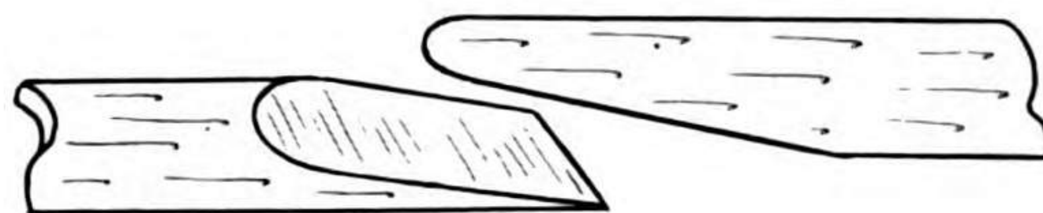
115. Ends of Edge Lacing Skived and Ready to Be Cemented
