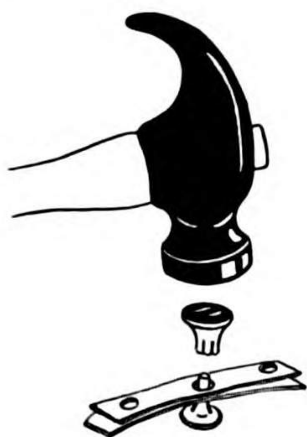
142. Setting a Rapid Rivet Cap on the Post
