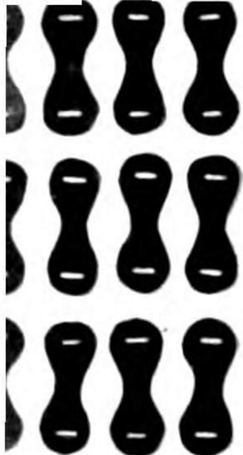
194. Utilizing Scrap Leather for Belt Links
