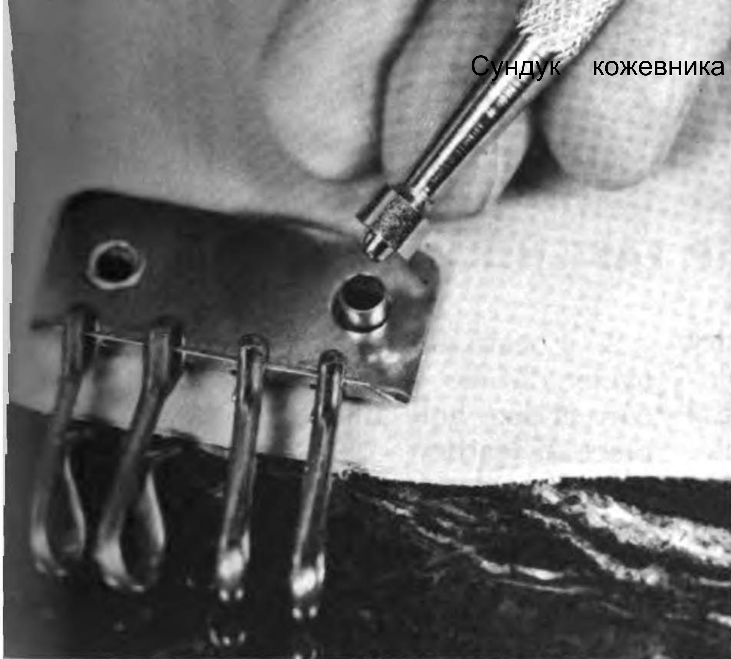
136. An Eyelet in Place Ready to Be Fastened or Secured with a Hand Eyelet Setter
