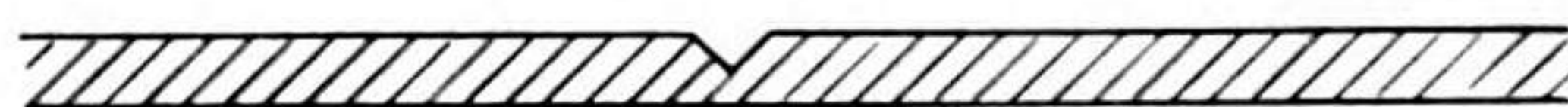
153. Detail of V Cut Showing Depth
