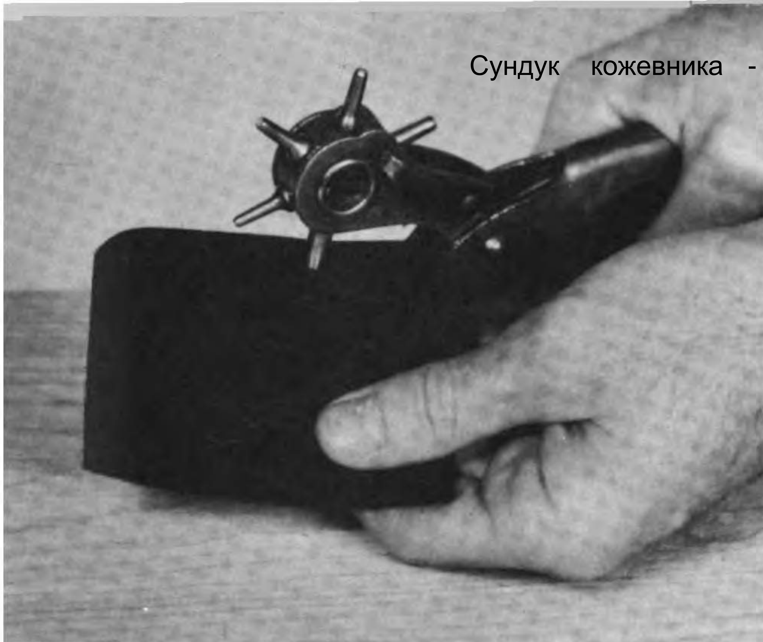
132. Punching a Hole with a Revolving Tube Hand Punch
