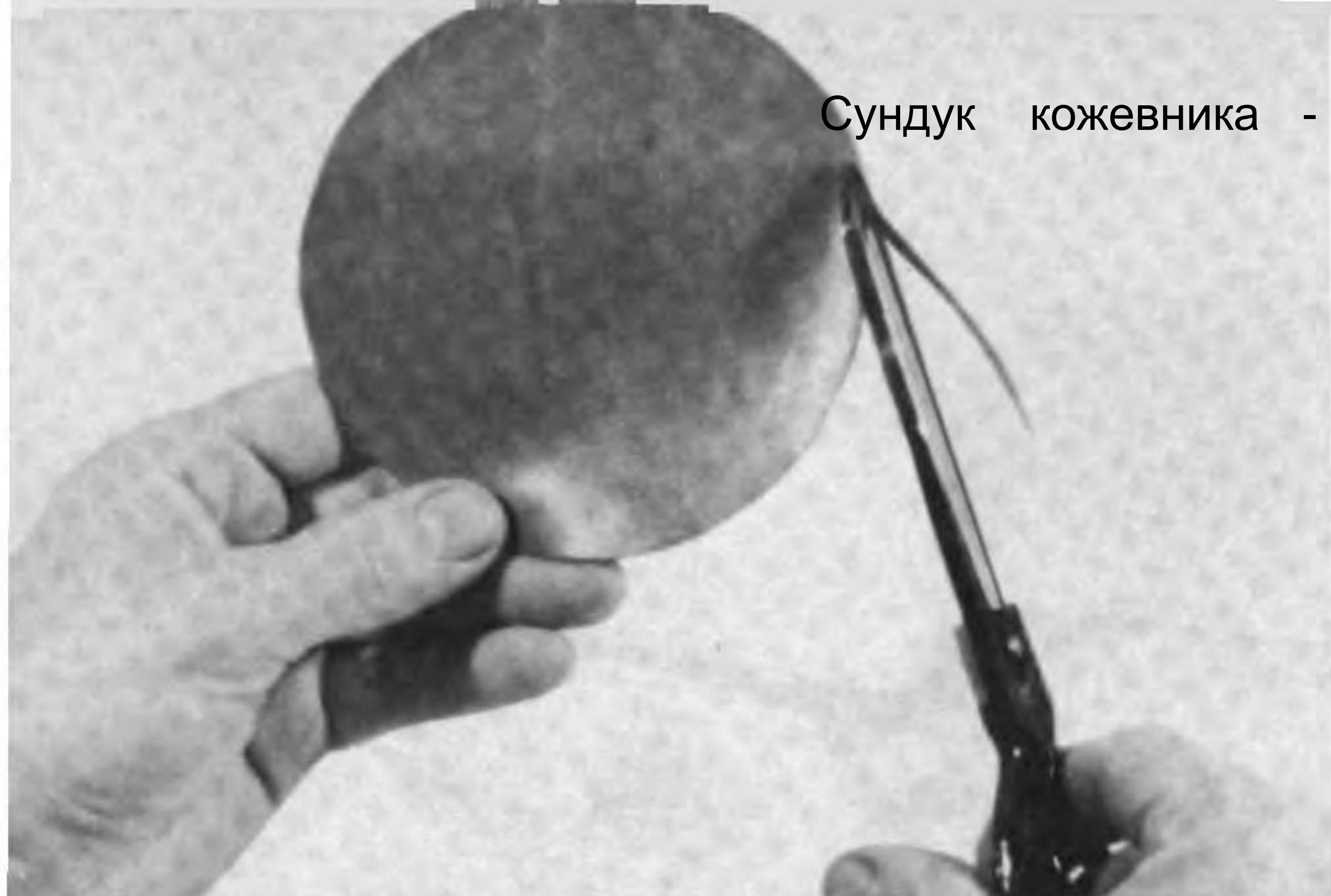
171. Cutting the Leader Strip on a Disk of Tooling Calf for Making Thong
