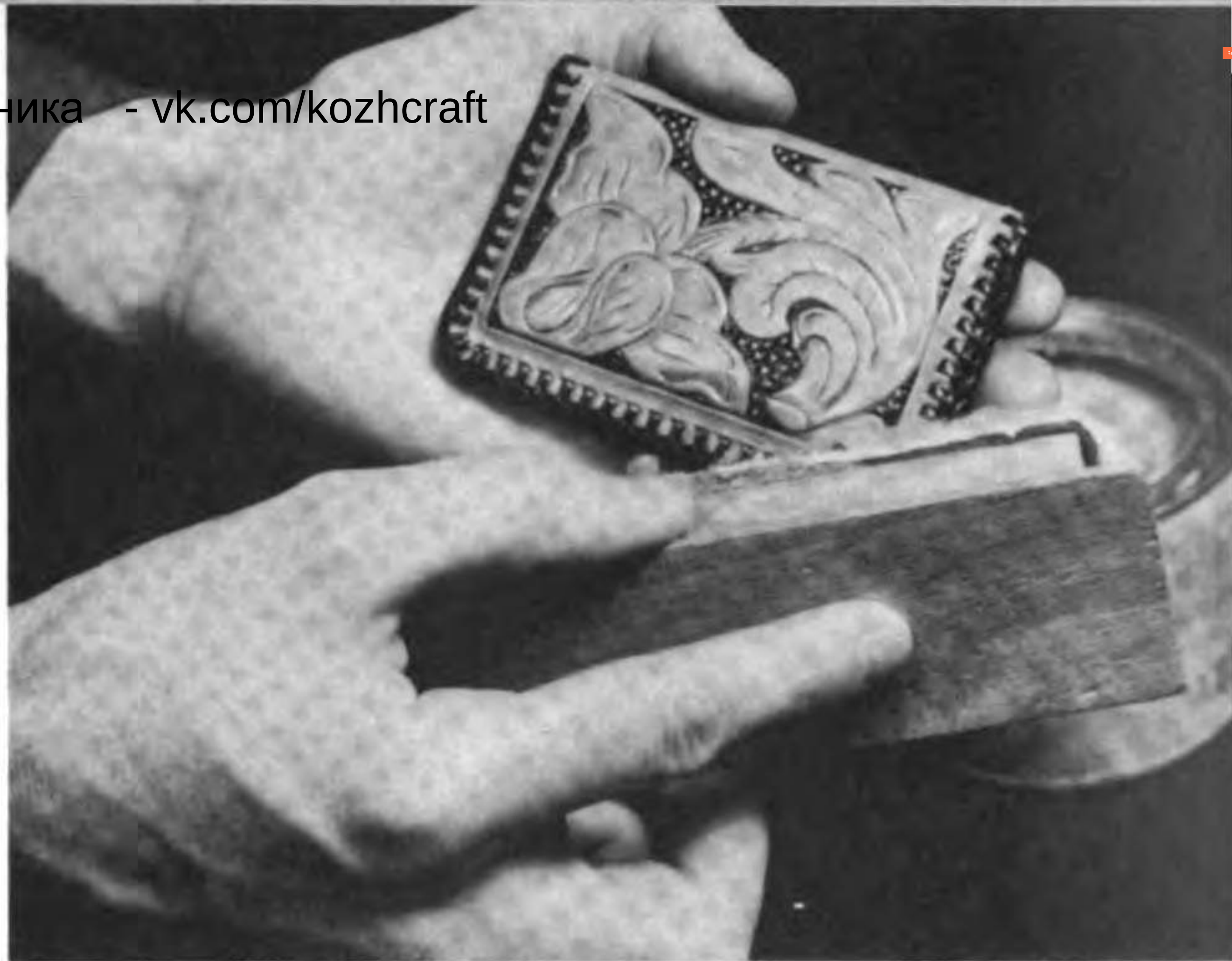
161. A Waxed Surface May Be Polished with a Hand Sheepskin Buffer
