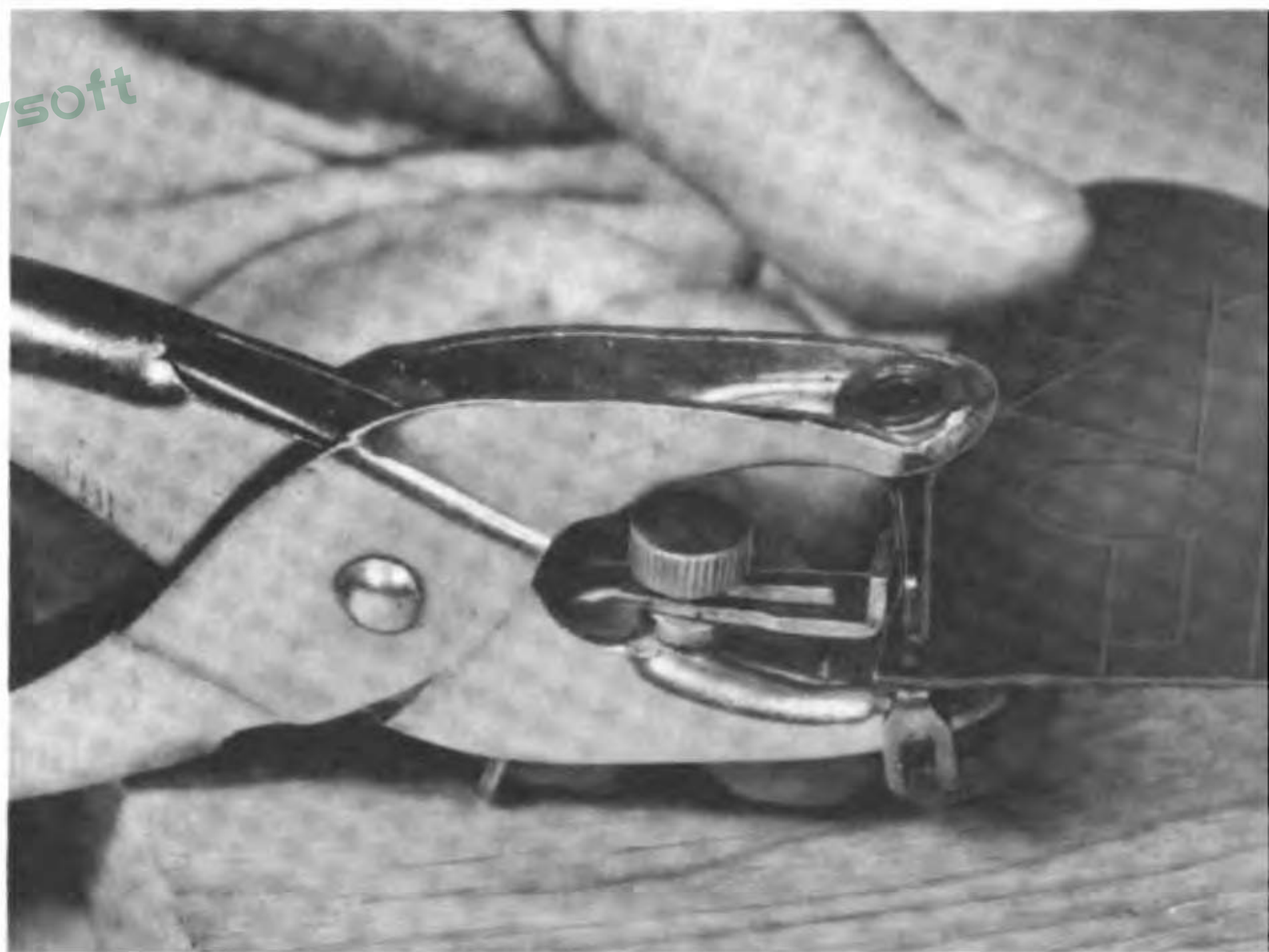
114. Making Edge Holes with Single Tube Punch. Note Depth and Spacer Gauges
