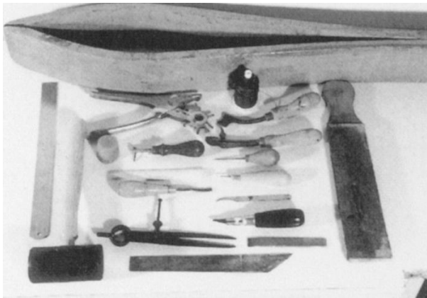
Fig 1 Basic tools: (top) clam; (left) ruler and rawhide mallet; (right) sharpening strop; (middle - clockwise from top) thread, step creaser, adjustable creaser, scratch awl, stitching awl, curved blade for clicker knife, clicker knife with straight blade, pricking iron, skiving knife, dividers, edge beveller, bone folder, stitching groover, beeswax, revolving punch-pliers.
