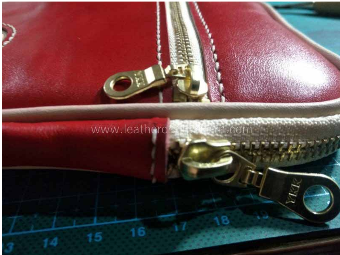
Step 18: Install zipper slider and sew zipper with gusset to finish this bag.
