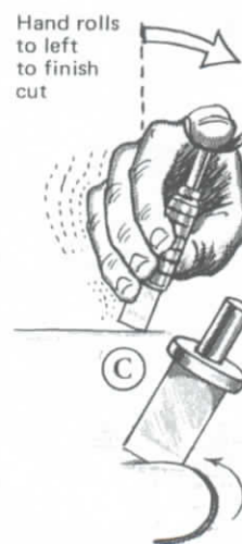
FRONT VIEW: showing position of hand and blade for cutting the left side of a circle.
