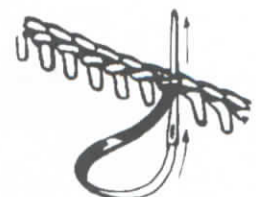
24: Push needle through the last hole as shown. Bring it up between the leathers and out between the lacing. Cut off the excess lace.
