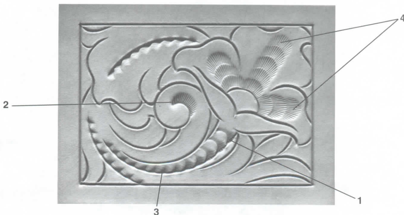
Photo above shows by number tool impressions created by the camouflage tool of corresponding number in the illustrations at top of the page.
