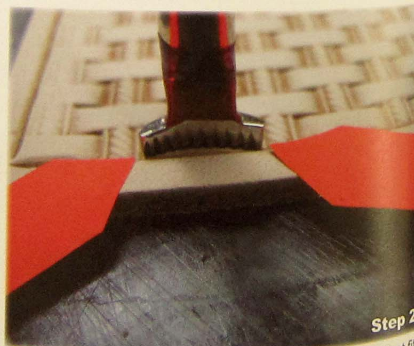
Step 2: For this design, you need to use a veiner tool that fits between the cross bars on the basket stamped design.
